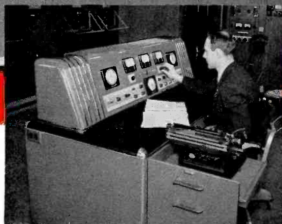
The operating console for the 50-kw transmitter provides single push-button starting for the entire transmitter with automatic sequence. Controls and indicator devices are provided for all major operating functions.
